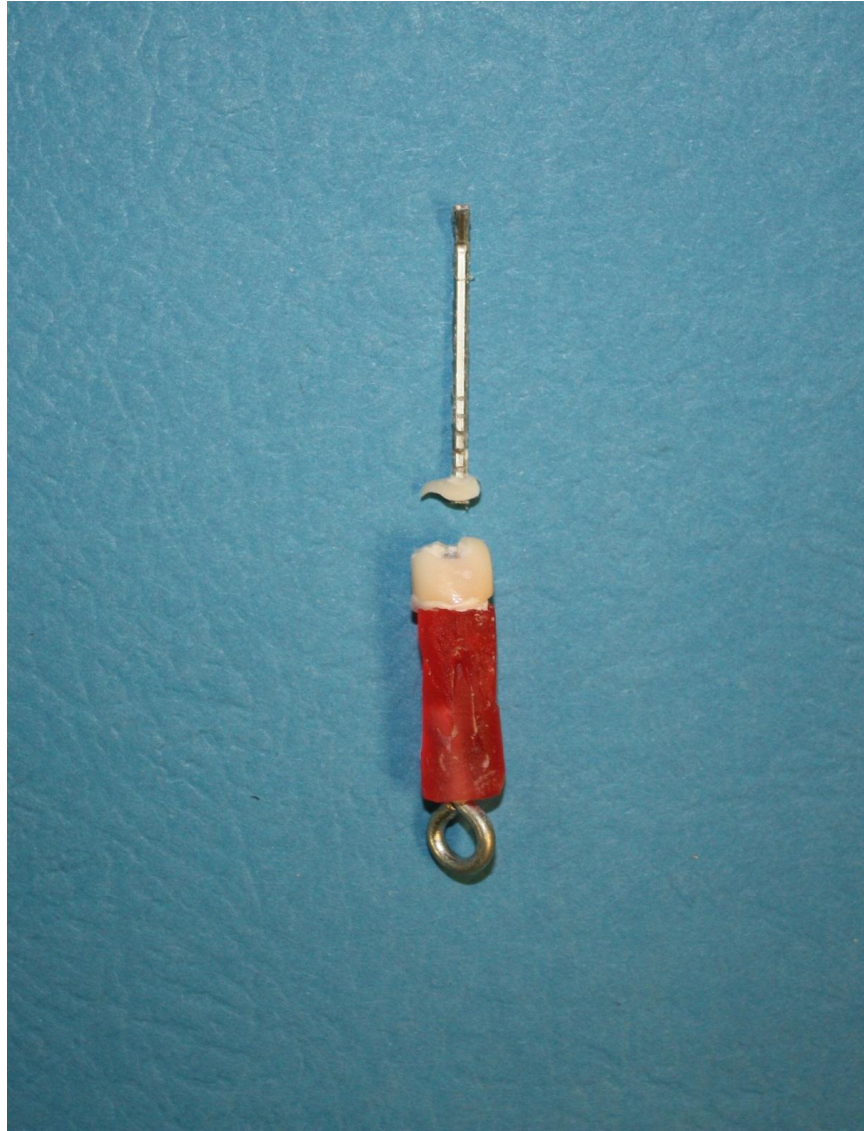
Figure 10 – EZ-Pedo – Ketac Cem – Porcelain Failure
