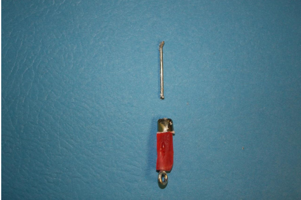
Figure 8: 3M Unitek – GC Fuji I - Nail Failure
